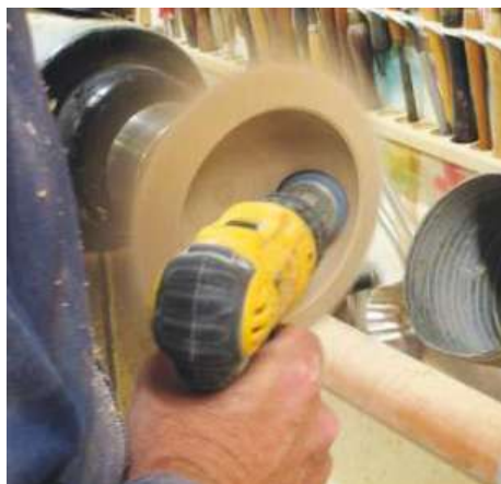
▲ Pic.32 You may find power sanding the interior difficult. I used a cordless drill for safety and this 3 o'clock position kept everything out of the way. Sand the edge with a block with the lathe switched off
